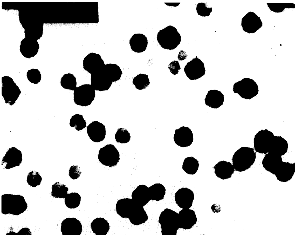
Fig. 1. Transmission electron micrograph of nanoparticles stained with PTA. Magnification 90,600\times .
